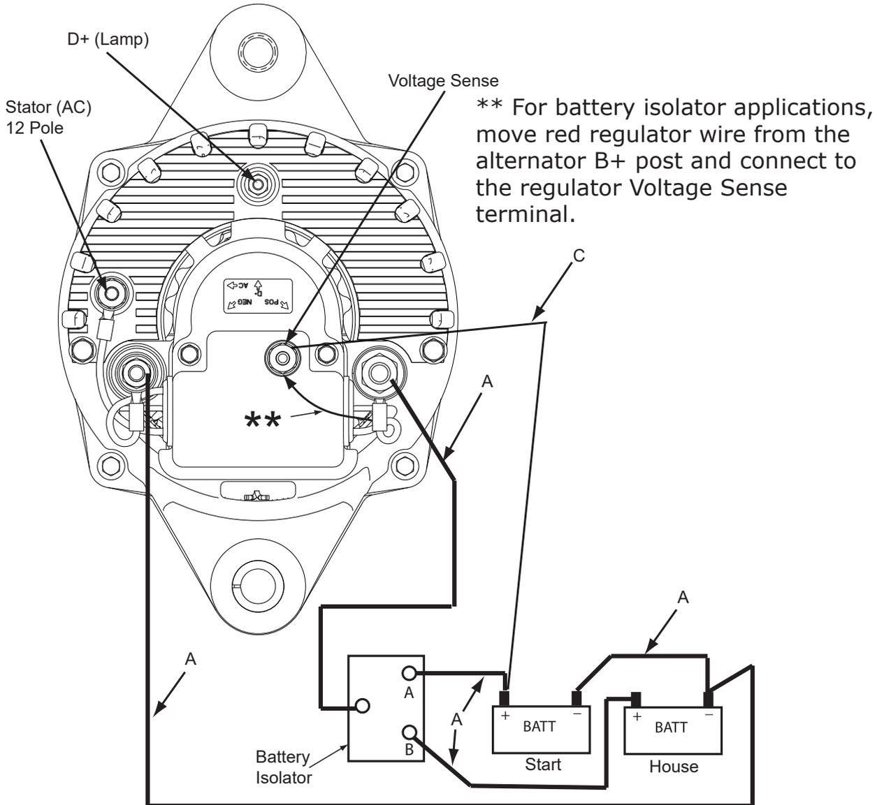
Note: If connection to remote sense terminal is lost, voltage will rise to approximately 30.5V. Connection to the remote sense terminal is mandatory.
