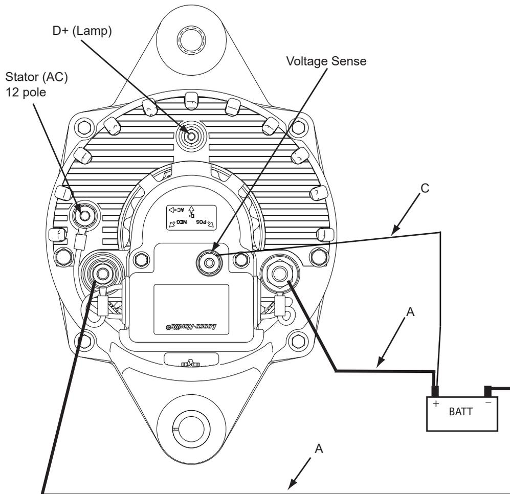
Note: If connection to remote sense terminal is lost, voltage will rise to approximately 30.5V.
